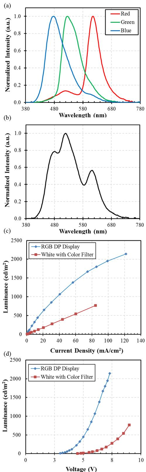
**Figure 7.** (a) Red, green, blue and (b) all pixels on spectra of an actively driven DP RGB AMOLED microdisplay. (c) J-L and (d) V-L comparison of DP RGB and conventional white with color filter AMOLED.
