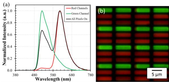
**Figure 4.**(a) Emission spectra for dual color display. (b) Optical microscope (63X) image of emission with all pixels on from directly patterned dual color display.
