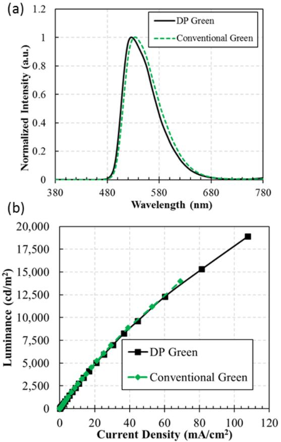
Figure 3. (a) Emission spectrum and (b) J-L characteristics of DP and conventional monochrome green AMOLED
