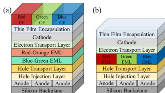
**Figure 1.** Structure of (a) conventional white OLED with color filter (CF) array in comparison with (b) directly patterned OLED with red, green and blue emitter layers (EML) eliminating the need for color filters.
