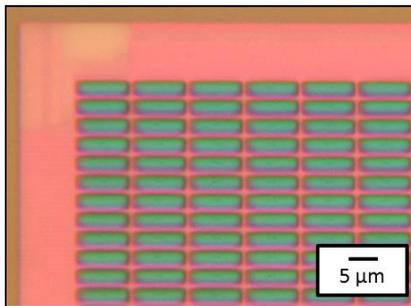
Figure 2. DP green emitter on WUXGA pixel array.
