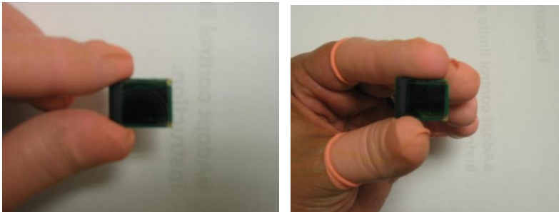
Fig. 3 Best method of handling the displays
