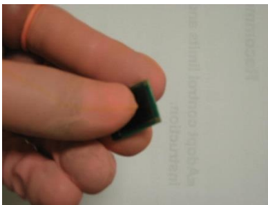
Fig. 4 Avoid this method of display handling
