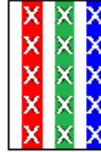
Example of 3 out/off sub-pixels = 1 pixel out
