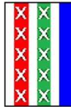
Example of a 2 sub-pixel out/off = Reject
