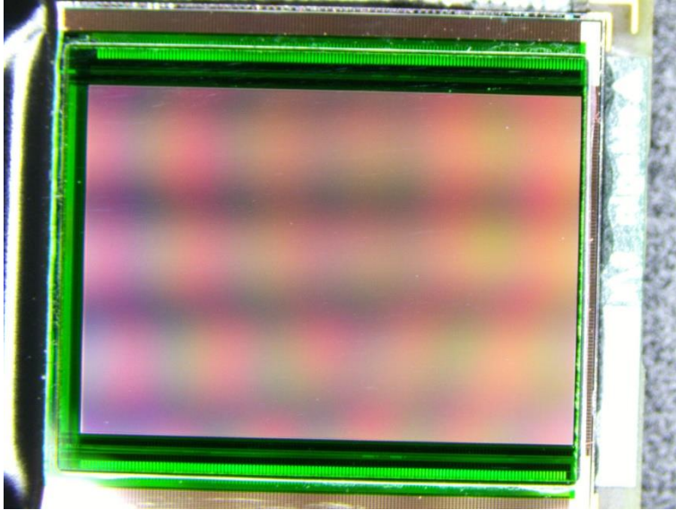
Edge of glass too close to the active area
