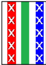
Example of a 2 sub-pixel out/off = Reject
