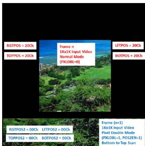
Figure 5. Transition from 1K1K native display to pixel doubled display
